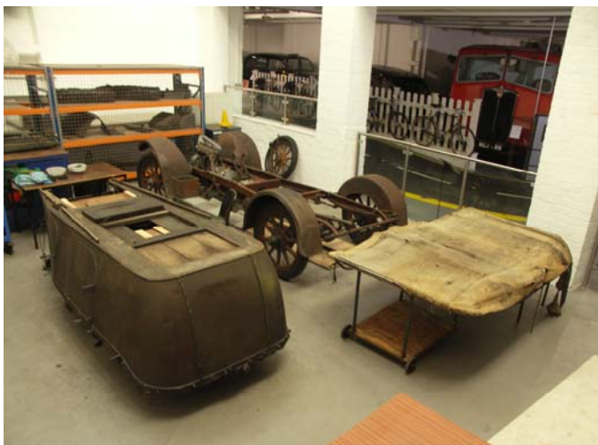
New workshop: the chassis, body and hood assembly making up the parts of the 1914 Humber 11 are suitably presented as a display for visitors
