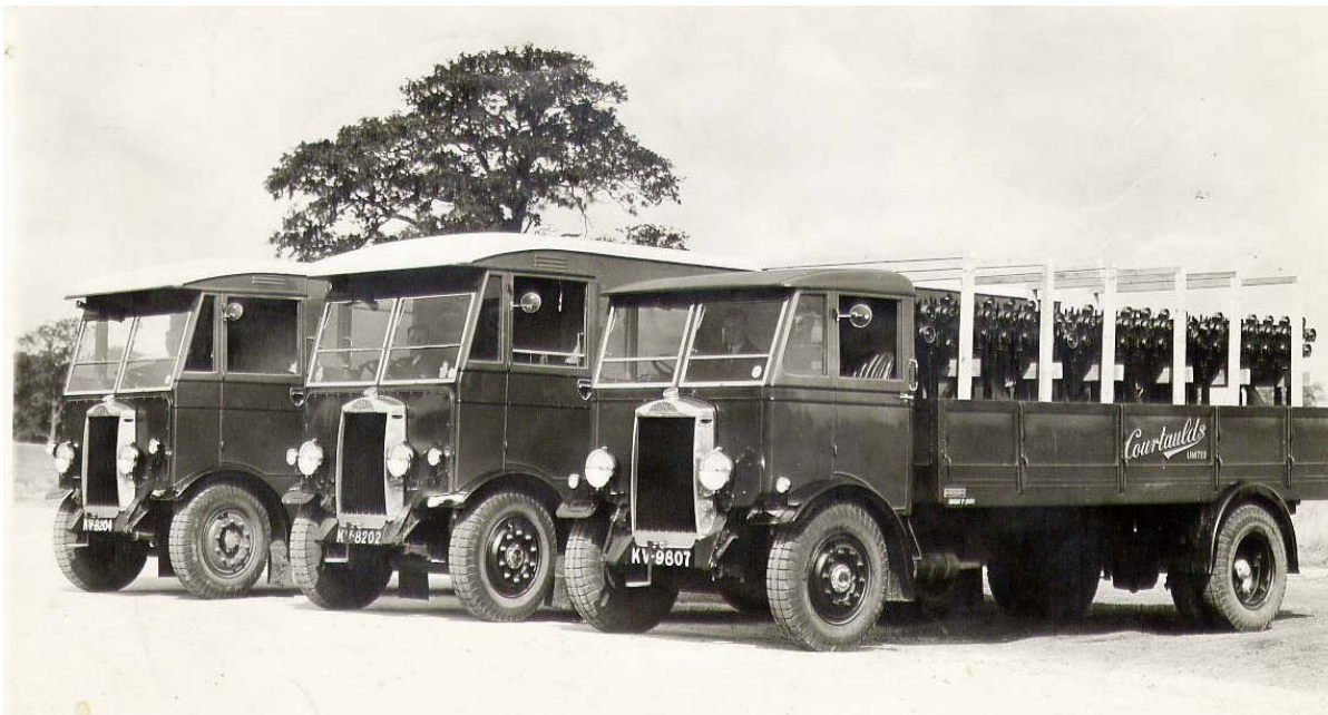
Line-up: Three Maudslay commercials that joined the Courtauld's fleet in 1933. They are believed to be the Six-four model that was brought out around 1930. KV 9807 appears to be equipped for carrying sections of machinery for the company's spinning process. The other two vehicles have been fitted with pantechicon bodywork.
